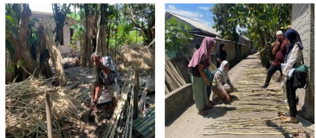
Figure 3. The process of manually making bamboo slats for blind products.
