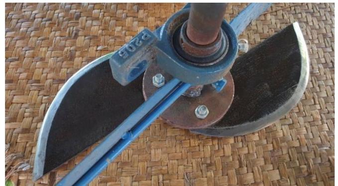
**Figure 5.** Chopping machine knife blade that had been sharpened
