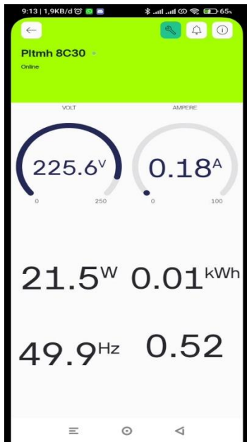
Figure 5. Real-time monitoring process in the application with IoT devices at the MHP in Argamukti Village
