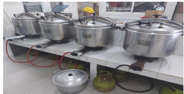
Figure 1. Conventional pressure cooker used by milkfish producers
