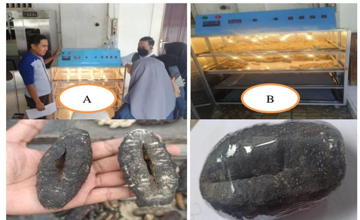
**Figure 3.** (A) Training on the use of ecoheat oven (B) Products inside the Ecoheat Oven (C) Products from sun drying (D) Products from ecoheat drying.
