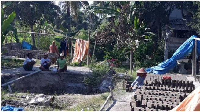
Figure 2. The drying process of molded red bricks, located at the business of Mr. Atahar
