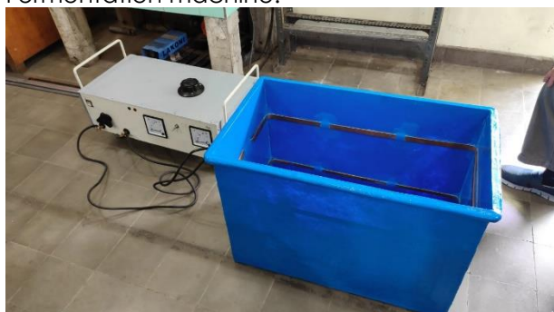
Figure 3. Arduino-Based Magnetic Fermentation Machine
