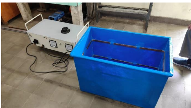
Figure 3. Arduino-Based Magnetic Fermentation Machine
