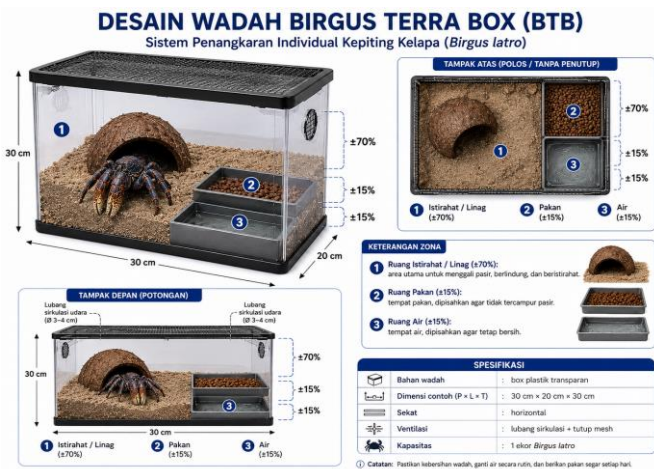
Figure 1. Functional schematic of the Birgus Terra Box (BTB) for individual coconut crab rearing, showing shelter/resting, feeding, and water zones, ventilation, and one-crab-per-unit capacity. Source: PKM Team design, 2026. Dimensions are illustrative and do not indicate that all field units were identical.
