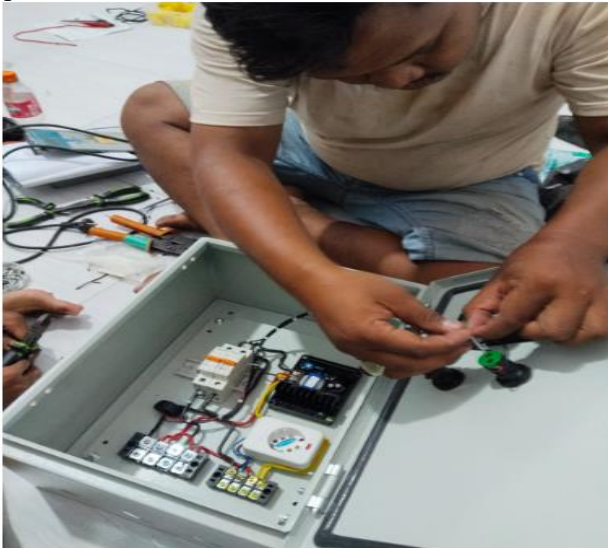
Figure 1. Presents The Design Of The Electronic Voltage Stabilizer Used In This Project
